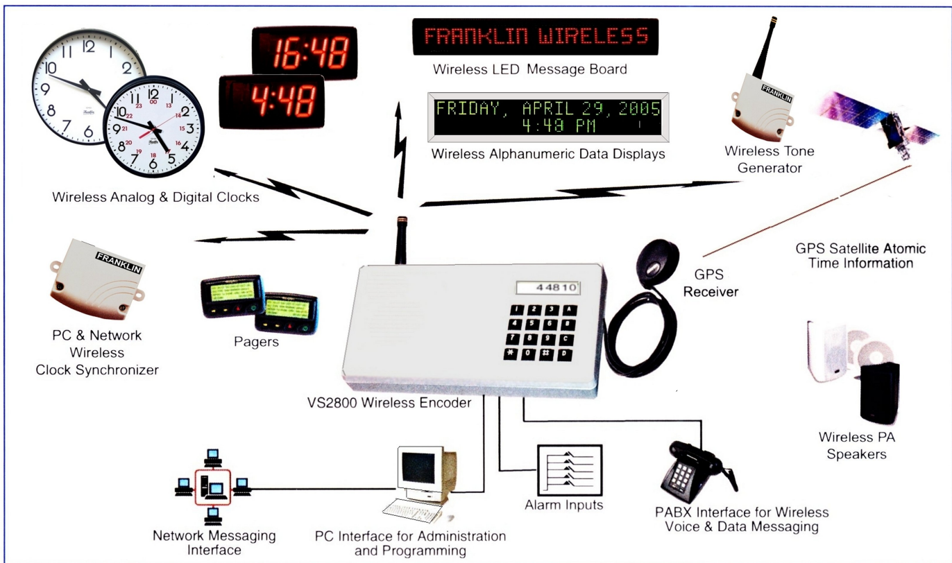
VS2800 Application Block Diagram
